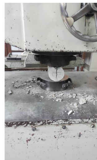
Figure 12: Split-tensile test 3. Results
