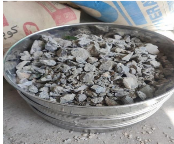
Figure 5: Screening of RCA through sieves)
