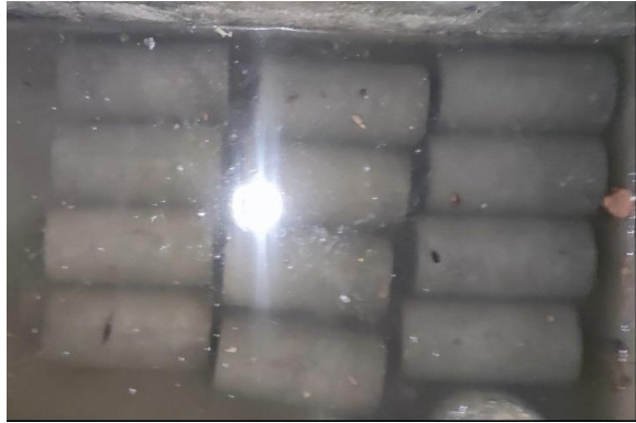
Figure 9: Specimens in the tank for curing
